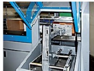
Servo-powered sealing ram forms square cases
