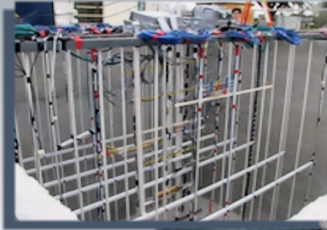
The sensing network in the open monolith (above), and after the curing stage (right).
