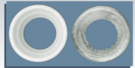
A Seal Showing Before / After of Radiological Degradation
