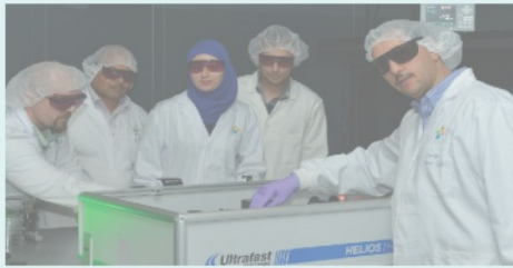
Prof. Omar Mohammed and his research team work in the laser lab at KAUST's Solar Center to align the femtosecond transient absorption setup to monitor electron injection between quantum dots (QDs) and phenyl-C 61 -butyric acid methyl ester (PCBM) in real time.
